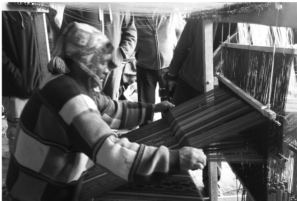
Figura 6. Telar a pedal
